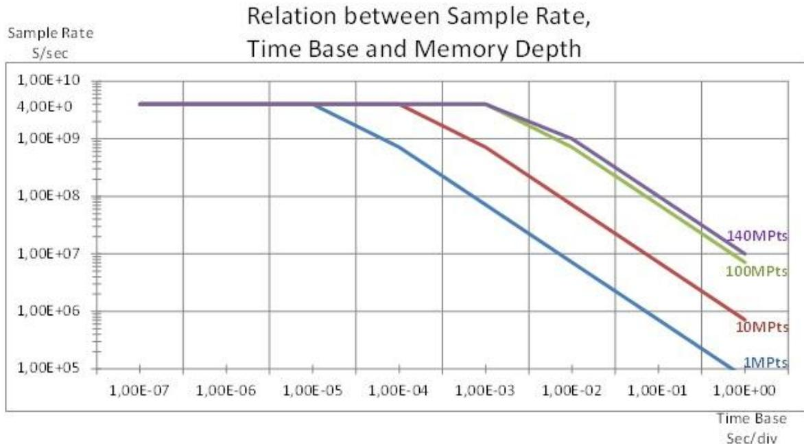
The graph also shows the influence of using different memory depths. As you can see, Larger memory depths allow you to maintain the maximum sample rate at longer time base scales. This provides more detailed waveforms over longer time spans.
