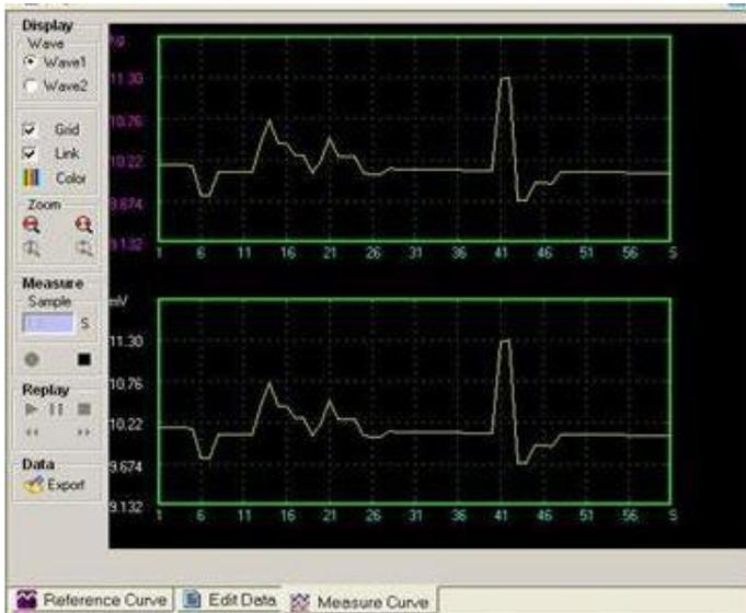
The last window is the Measure Curve. Here the real time measured waveform of the Digital Multimeter is displayed. The waveform can be replayed after it has been recorded and it can also be exported as a \*.txt or \*.csv file and so used as a future reference curve.
