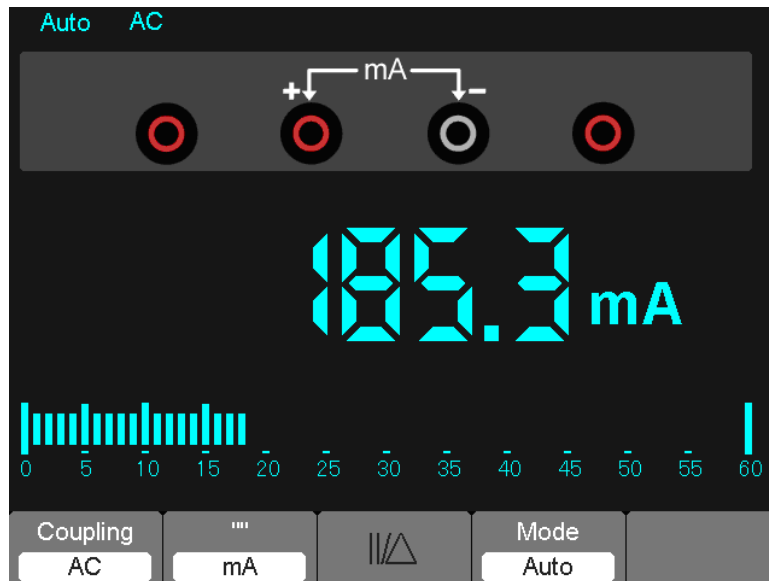
Figure 7-10 AC Current Measurement for 600 mA
