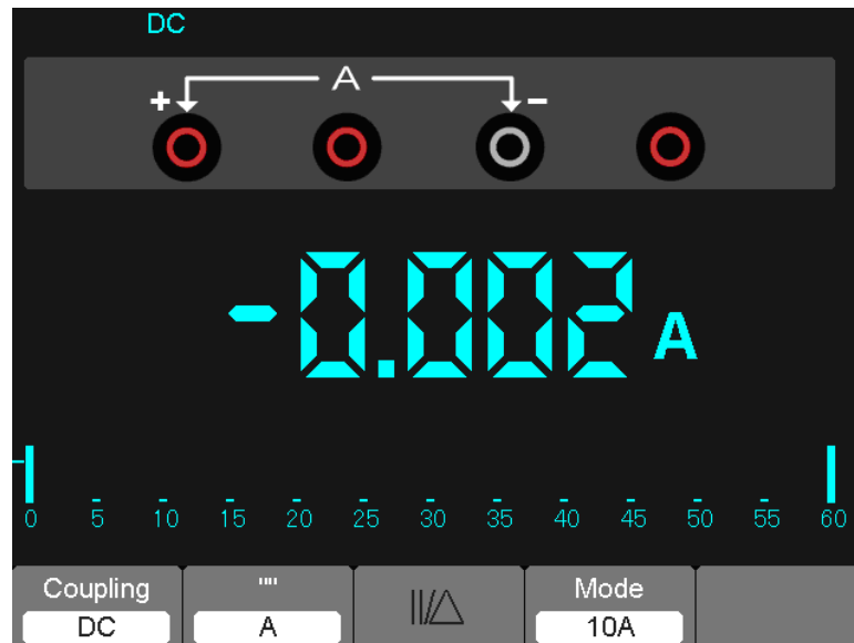
Figure 7-9 DC Current Measurement for 10A
