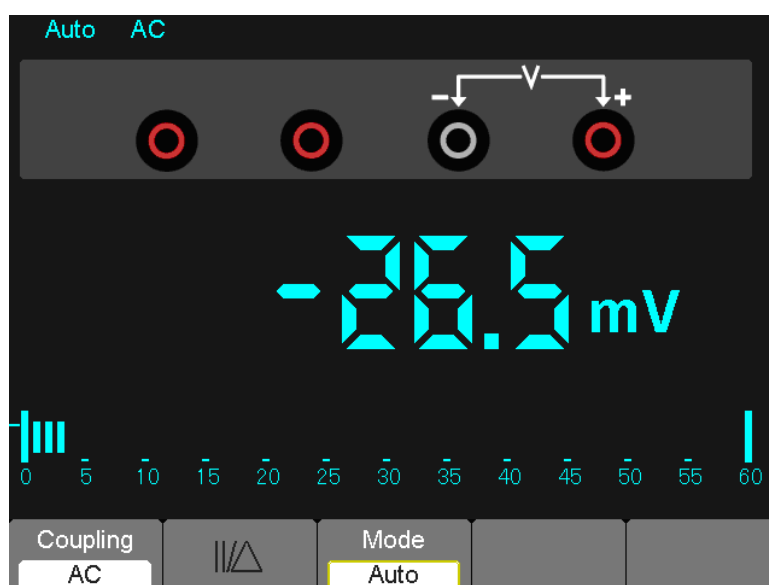
Figure 7-7 AC voltage Measurement
