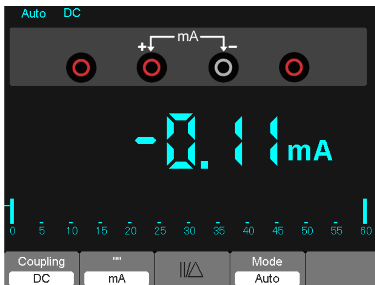
Figure 7-8 DC current Measurement for 600 Measurement
