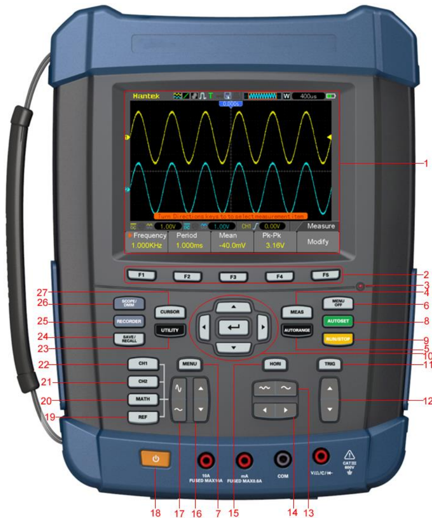
Front Panel of DSO1000E Series
