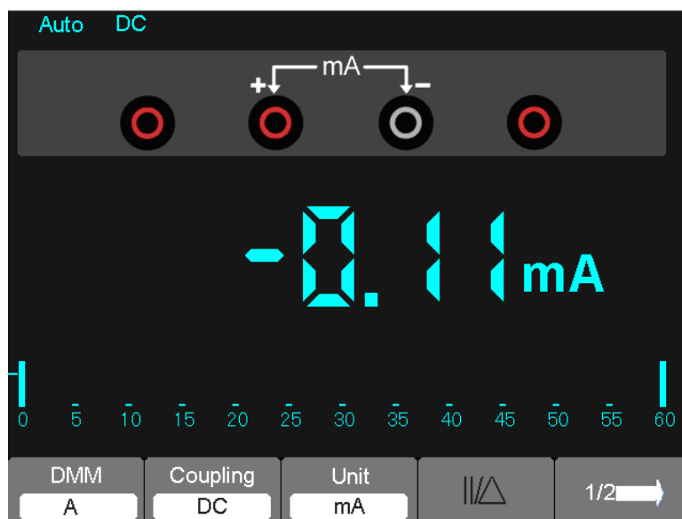
Figure 7-8 DC current Measurement for 600 Measurement
