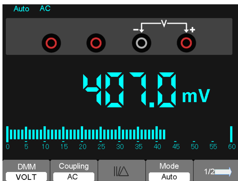
Figure 7-7 AC voltage Measurement
